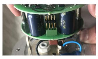
Modules and components include protective elements that prevent incorrect assembly
