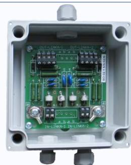
Module BO-02 - overvoltage protection of two independent transmission lines of system DAP 128TC
